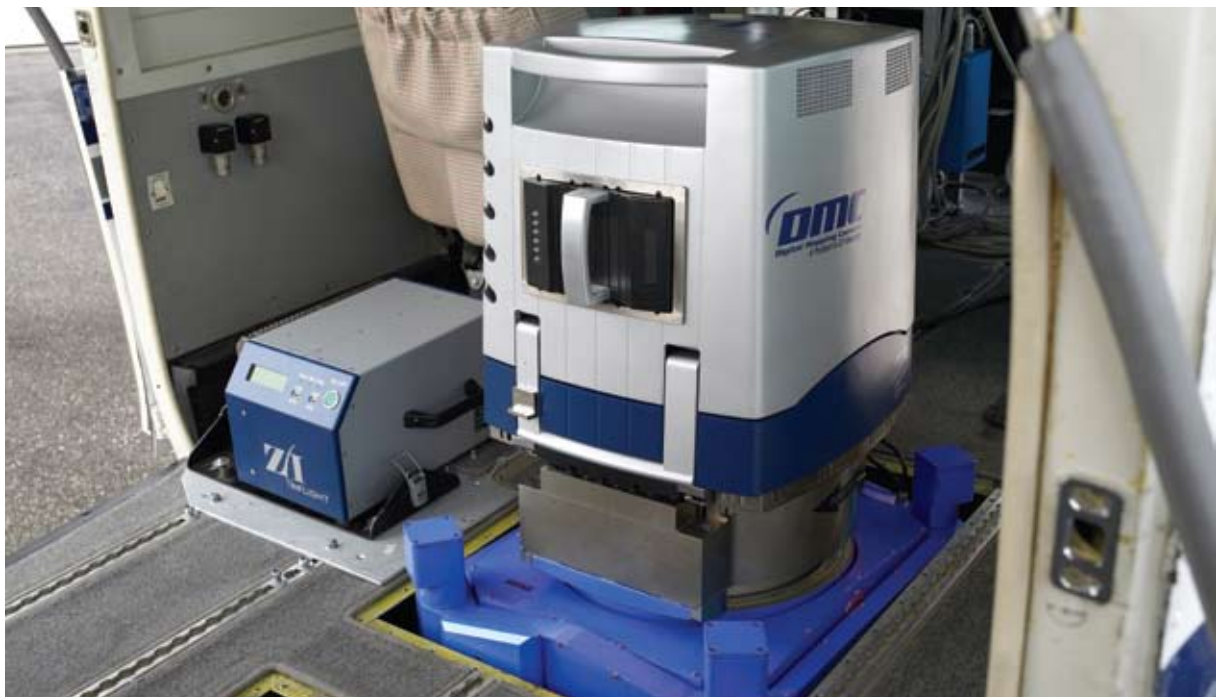
The DMC's solid state disk technology has the capacity to store 1,200 images in a single cartridge.
